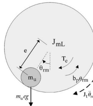
Figure 1. Rotational unbalanced model of the motor [7]
