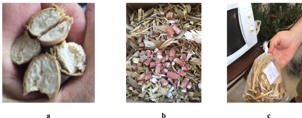
Figure 3. Close-up view of the cellulosic stem tissue of the stalk section of maize harvest residues, b) the mixture of harvest residues after the shredding process, and c) sample prepared and labeled for applications.
