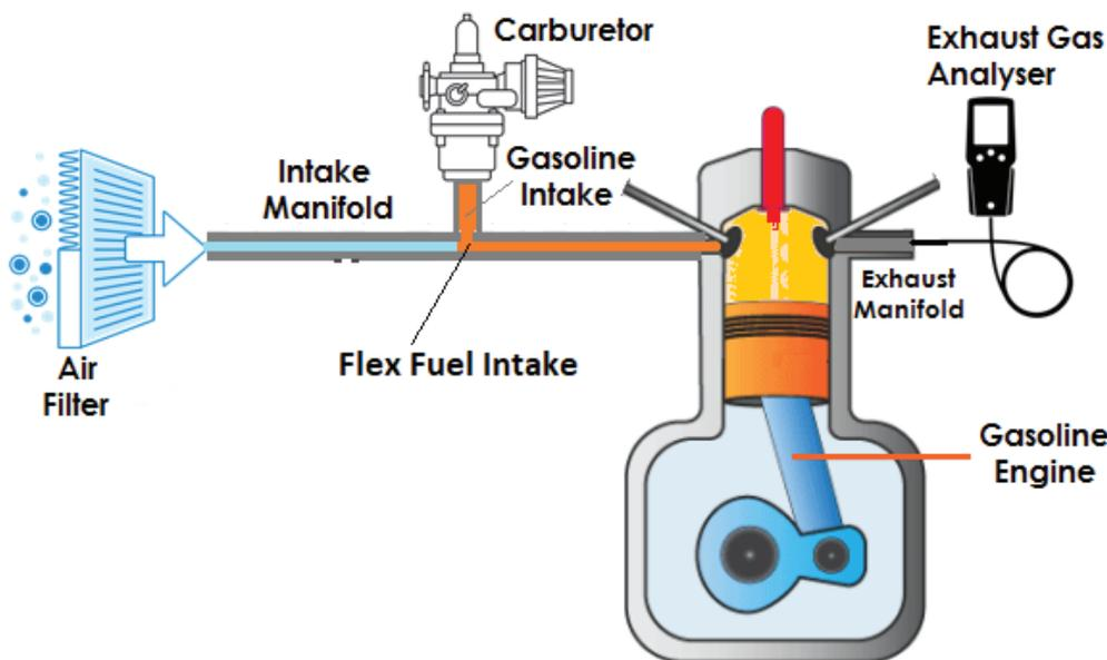
Figure 1. Schematic diagram of the Bio-ethanol Setup [14].
