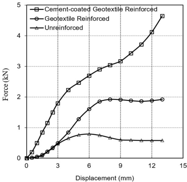
Figure 5. Force-displacement curves for sand soil
