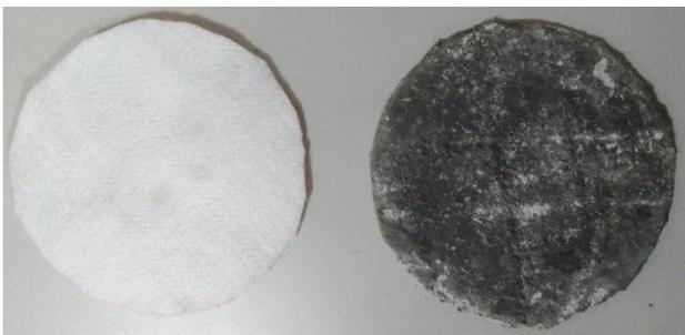
**Figure 2.** The photograph of geotextile and cement-coated geotextile
