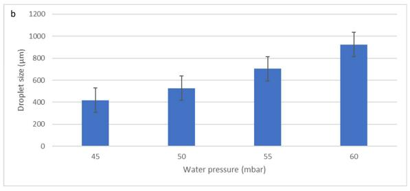
Figure 3 Water in oil droplets in a microchannel (a) Microscope photo microdroplets inside the channel for several water pressures. (b) Droplet size across water pressure.
