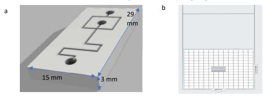
Figure 1 (a) View of the microchannel in CAD file (b) microchannel directly placed over the build platform in Preform software.
