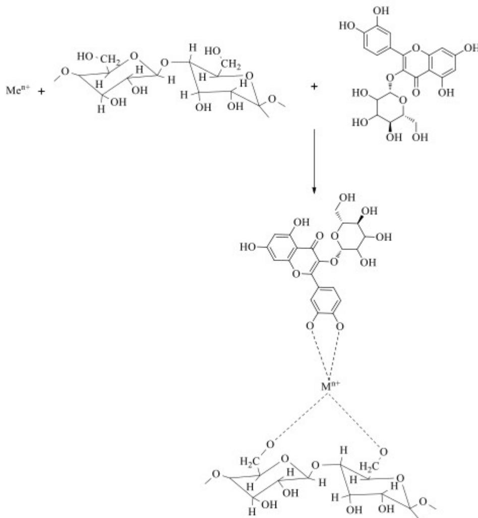
**Figure 3:** The proposed mechanism of dyestuff with mordants for cotton fabric.
