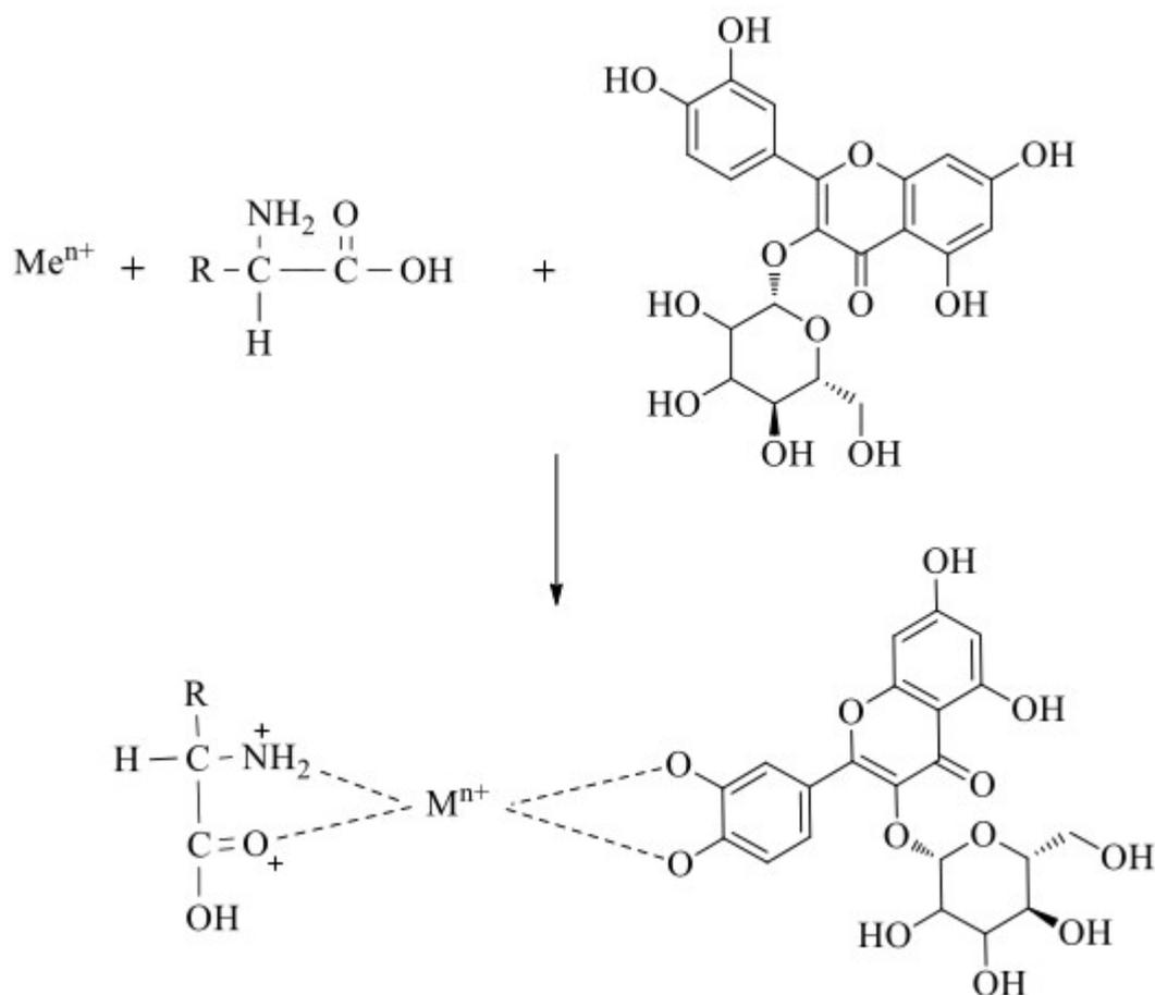
**Figure 2:** The proposed mechanism of dyestuff with mordants for wool yarn.
