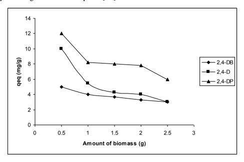
**FIGURE 3** Effect of amount of biomass on equilibrium bisorption capacity (initial pesticide concentration ( $C_o$ ) = 10 mg/l, pH 6.0, contact time 60 min, temperature (T)= 25  $^{\rm O}$ C)
