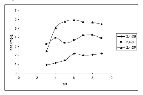
**FIGURE 2** Effect of pH of the solution on equilibrium bisorption capacity (initial pesticide concentration  $(C_o) = 10 \text{ mg/l}$ , contact time 60 min, temperature  $(T) = 25 \text{ }^{O}C$ , biosorbent amount (m) = 2 g)
