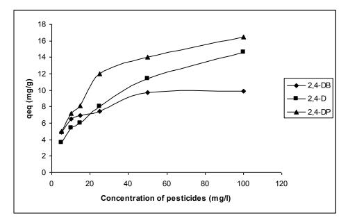
**FIGURE 4** Effect of initial pesticides concentration on equilibrium bisorption capacity (pH 6.0, temperature (T)=  $25^{\circ}$ C, biosorbent amount (m)= 2 g, contact time 60 min)
