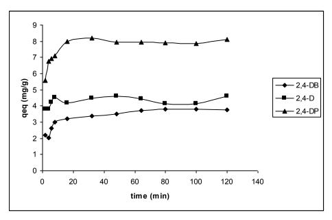
**FIGURE 1** Effect of contact time on equilibrium bisorption capacity (initial pesticide concentration  $(C_o) = 10 \text{ mg/l}, \text{ pH 4.0}, \text{ temperature } (T) = 25 \text{ }^{O}\text{C}, \text{ biosorbent amount } (m) = 2 \text{ g})$
