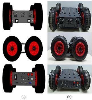
**Figure 3.** Mobile robot (a) 3D drawing view and (b) Realized view
