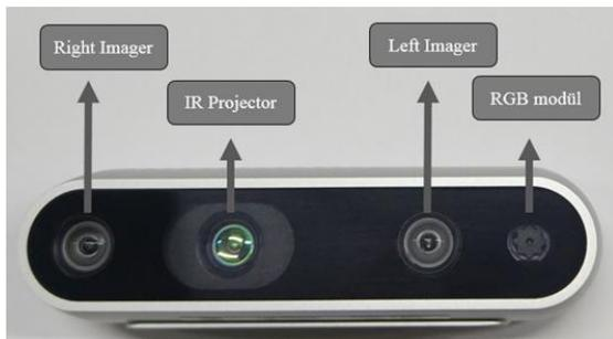
**Figure 1.** Intel® RealSense™ D435 Camera
