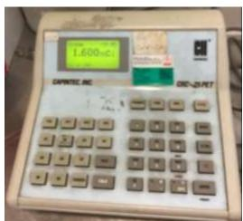
Figure 11. Low activity Technesium-99 at 20V
