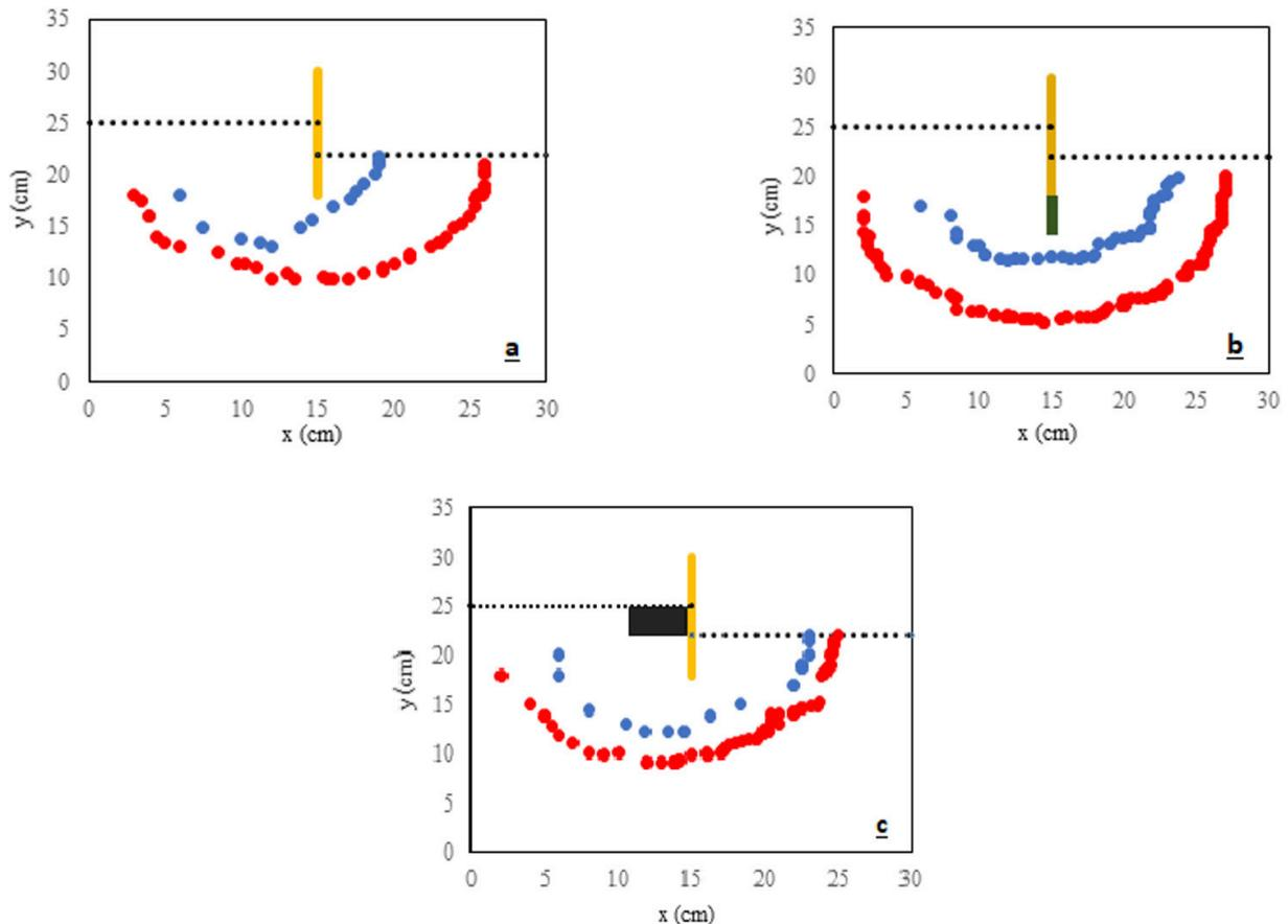
**Figure 4.** a) General b) Sheet pile c) Upstream clay blanket system test plots (for  $d_1=0.85\text{mm}$ )
