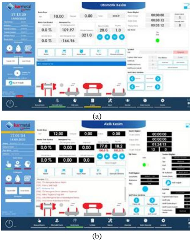
**Figure 4.** Operatorpanel interface (a) Smart cutting mode operator panel, (b) Automatic cutting mode operator panel
