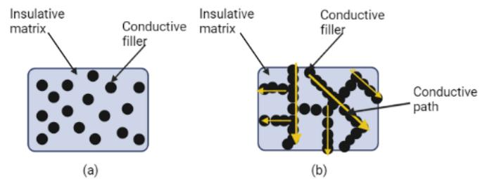
**Figure 3.** Schematic representation of filler distribution in polymer matrix, a) at low content, b) at high content [54].
