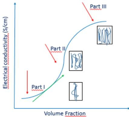
**Figure 4.** The dependence of electrical conductivity on the filler volume fraction [53]
