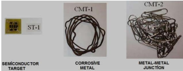
Figure 2: Semiconductor, corrosive metal and metal metal junction targets.
