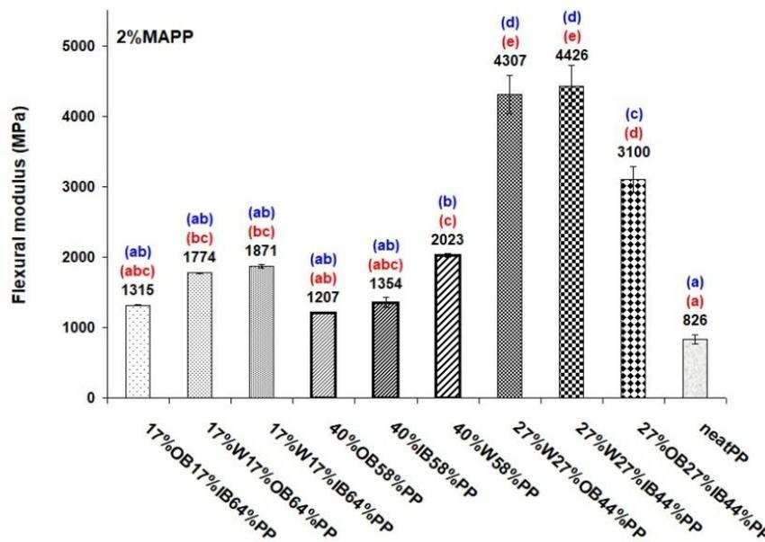
**Figure 2.** Mean values of flexural modulus of the IB/PP, OB/PP, W/PP, IB/OB/PP, IB/W/PP, OB/W/PP, IB/OB/W/PP and neat PP composites. Multiple range tests of Duncan that are indicated within parentheses demonstrate varying alphabetical designations highlighting significant differences among different treatments (composites). Red colour means at a 95% confidence level and blue colour means at a 99% confidence level.
