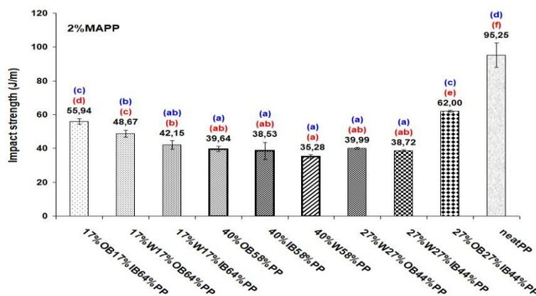
**Figure 5.** Mean values of impact strength of the IB/PP, OB/PP, W/PP, IB/OB/PP, IB/W/PP, OB/W/PP, IB/OB/W/PP and neat PP composites. Multiple range tests of Duncan indicated within parentheses denote distinct alphabetical designations underscoring significant disparities among various treatments (composites). Red colour means at a 95% confidence level and blue colour means at a 99% confidence level.
