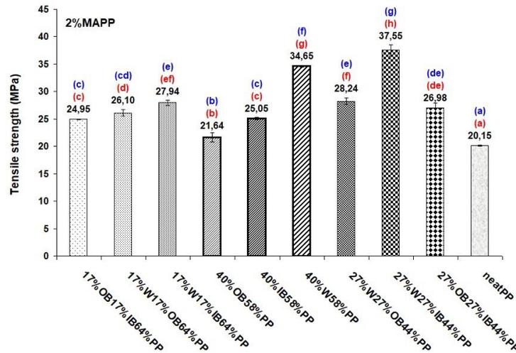
**Figure 3.** Mean values of tensile strength of the IB/PP, OB/PP, W/PP, IB/OB/PP, IB/W/PP, OB/W/PP, IB/OB/W/PP and neat PP composites. Multiple range tests of Duncan presented in parentheses signify distinct alphabetical designations that indicate significant disparities among various treatments (composites). Red colour means at a 95% confidence level and blue colour means at a 99% confidence level.
