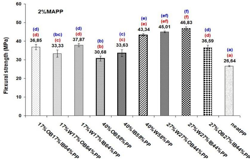
**Figure 1.** Mean values of flexural strength of the IB/PP, OB/PP, W/PP, IB/OB/PP, IB/W/PP, OB/W/PP, IB/OB/W/PP and neat PP composites. Multiple range tests of Duncan (in parentheses) reveal distinct alphabetical designations signifying significant differences among various treatments (composites). Red colour means at a 95% confidence level and blue colour means at a 99% confidence level.
