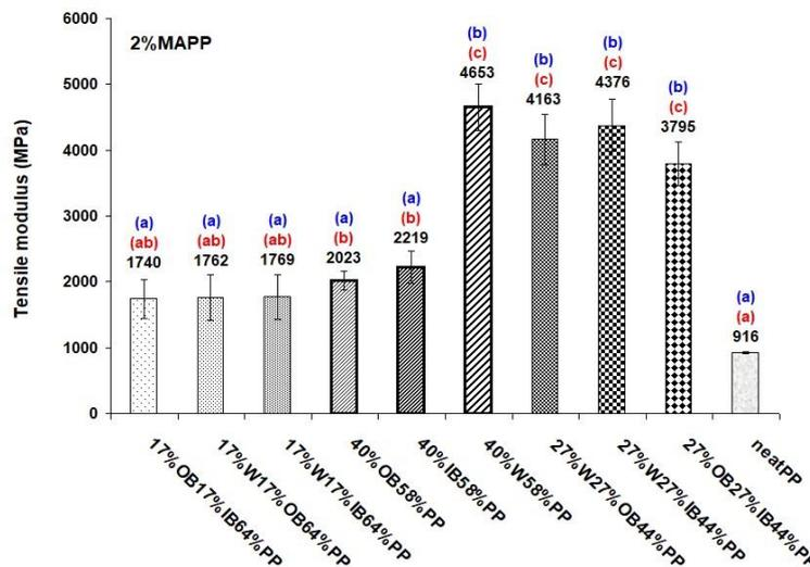
**Figure 4.** Mean values of tensile modulus of the IB/PP, OB/PP, W/PP, IB/OB/PP, IB/W/PP, OB/W/PP, IB/OB/W/PP and neat PP composites. Multiple range tests of Duncan presented in parentheses signify distinct alphabetical designations that indicates significant disparities among various treatments (composites). Red colour means at a 95% confidence level and blue colour means at a 99% confidence level.
