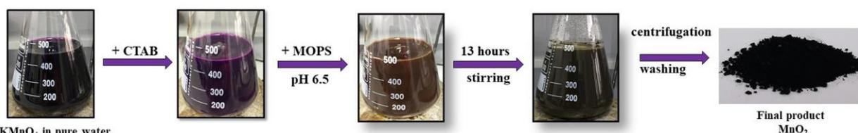
**Figure 2.** Synthesis of  $\text{MnO}_2$
