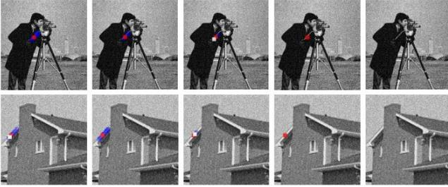
Fig. 2. The matching process of BM3D noise removal
