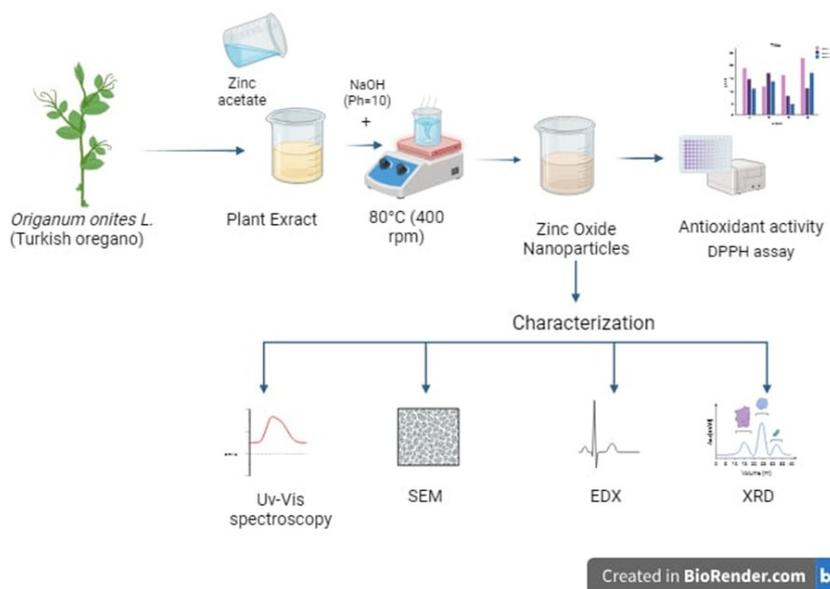
Figure 1. Biosynthesis of Turkish Oregano Zinc Oxide Nanoparticles (O-ZnO NPs)
