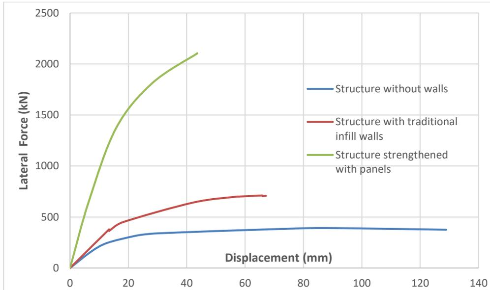
**Figure 14.** The force displacement curves of 3 story frames
