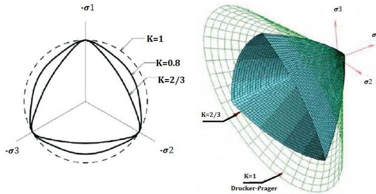
Figure 3. Demonstration of CDP model yielding surface [15]
