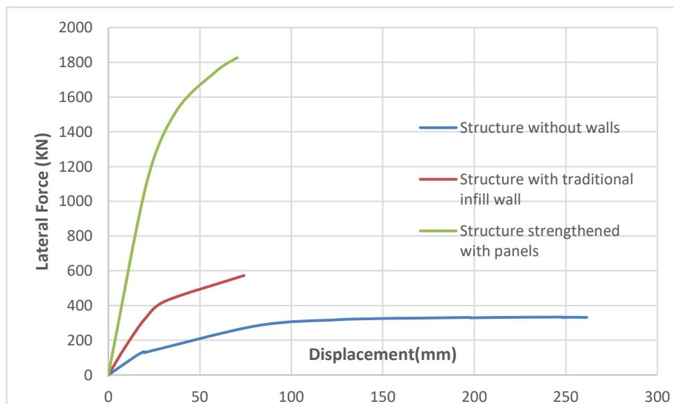
**Figure 15.** The force displacement curves of 5 story frames
