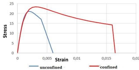
Figure 6. Mander model for defining stress-strain relations of concrete [24]
