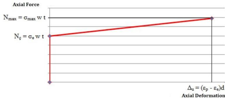
Figure 7. The axial force deformation relationship of nonlinear hinges in the middle of compressive struts [30]
