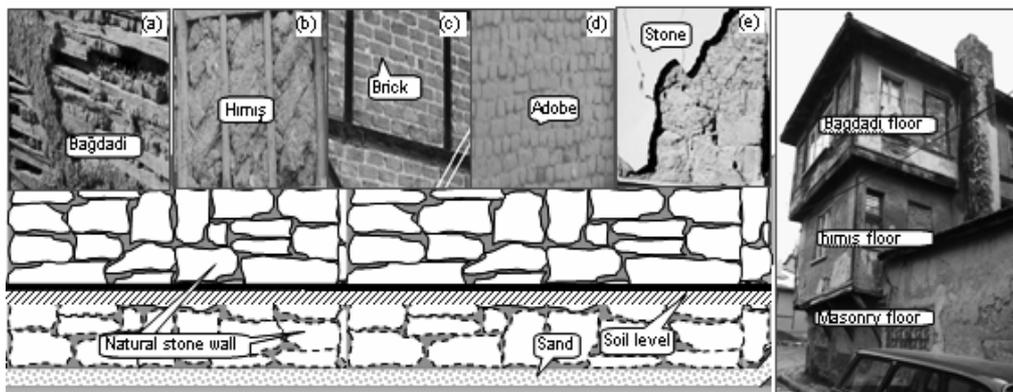
Figure 3. Systems of foundation and kinds of wall
