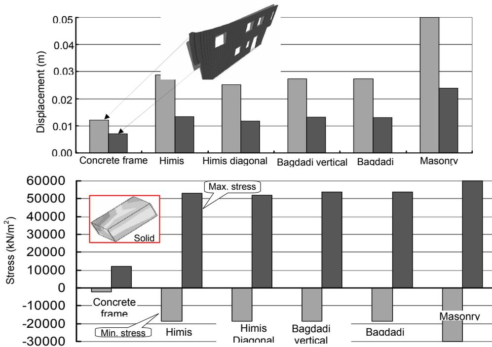
Figure 15. Displacements and stresses according to different types of structures
