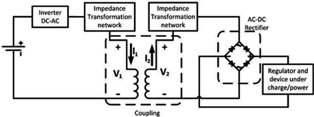
Figure 2. Typical near-field power transfer system structure.
