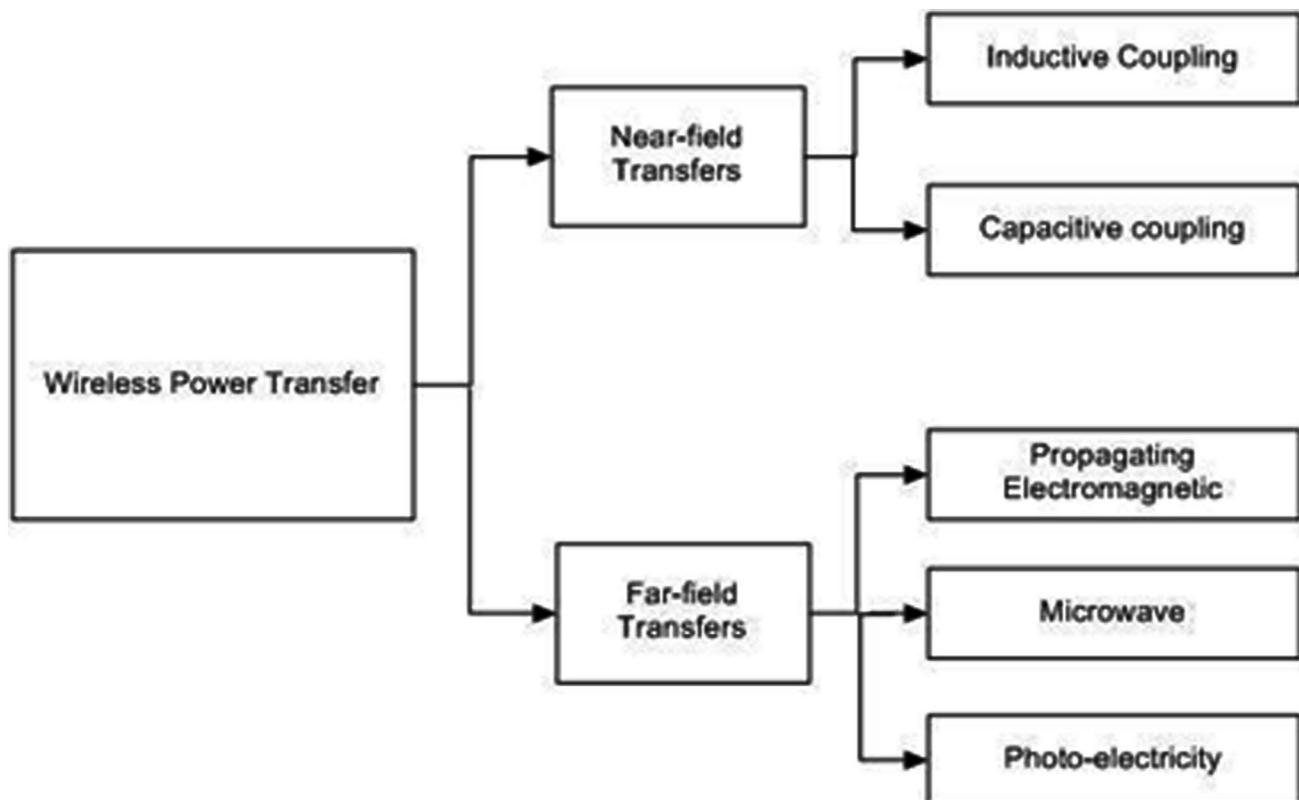
**Figure 1.** Wireless power transmission types.
