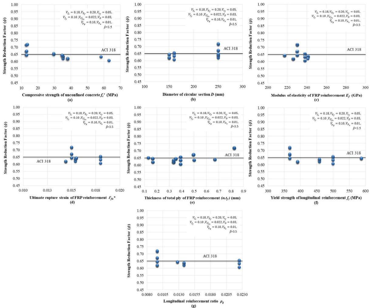
Figure 7. Strength reduction factors versus variables of the reinforced circular columns for case “23” and the target reliability index ( $\beta=3.5$ ) [44].
