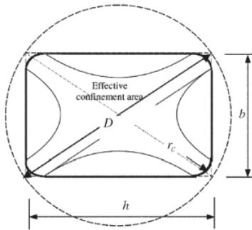
Figure 1. Equivalent circular cross section [3].
