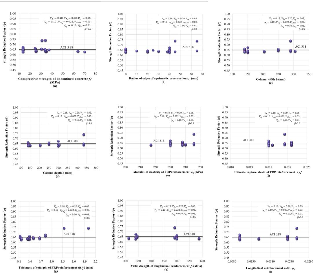
Figure 11. Strength reduction factors versus variables of the reinforced rectangular columns for case “23” and the target reliability index ( $\beta=3.5$ ) [44].
