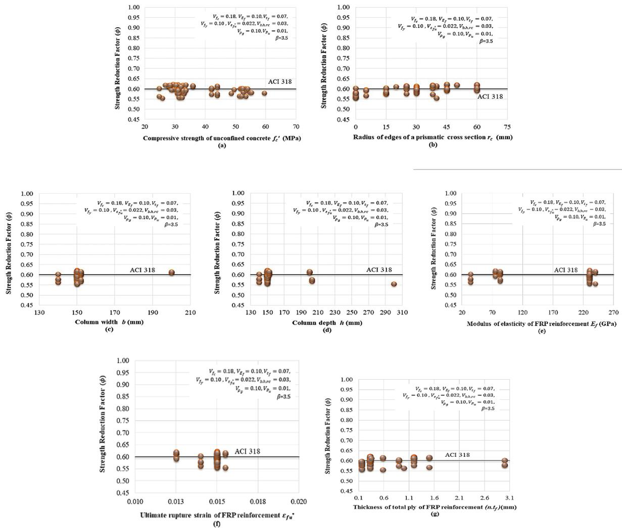
Figure 12. Strength reduction factors versus variables of the unreinforced rectangular columns for case “20” and the target reliability index ( $\beta=3.5$ ) [44].
