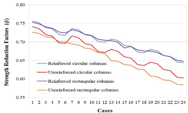
Figure 14. Comparison of the mean strength reduction factors for all column specimens [44].
