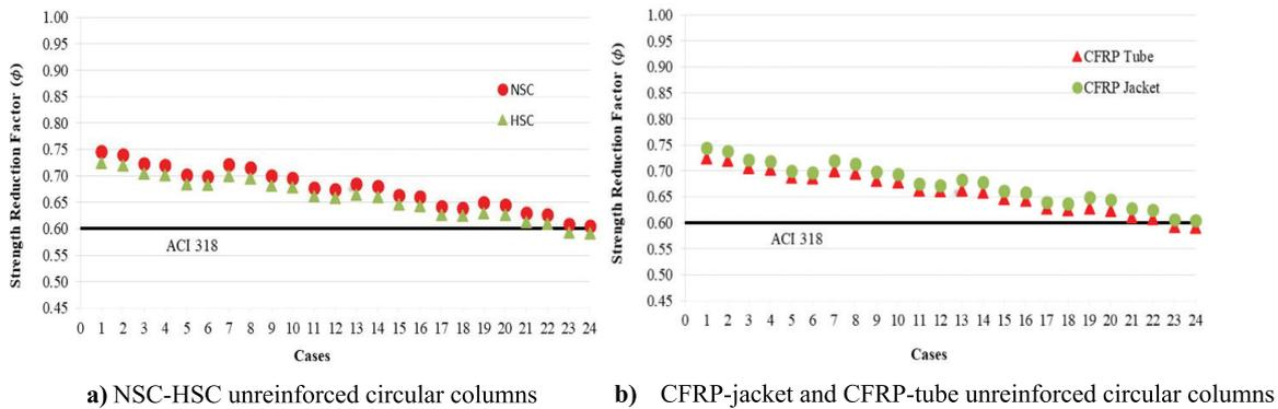
**Figure 9.** Comparison of the strength reduction factors of NSC-HSC and CFRP-jacket and CFRP-tube unreinforced circular column specimens for all cases [44].
