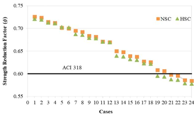
Figure 13. Comparison of the strength reduction factors for NSC and HSC unreinforced rectangular column specimens [44].
