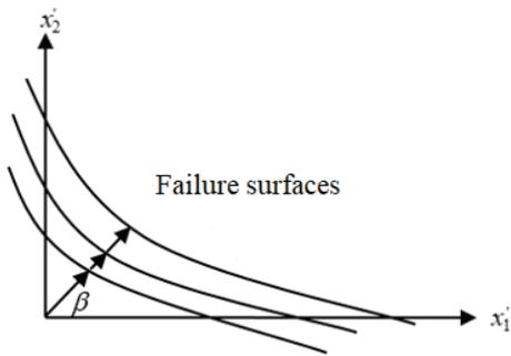
**Figure 3.** Designs corresponding to different failure surfaces [2].
