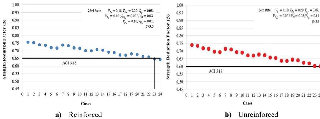
Figure 6. Distributions of strength reduction factor of reinforced and unreinforced circular test specimens [44].
