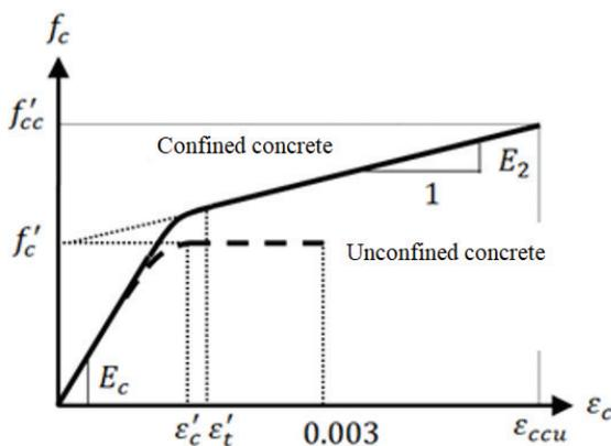
Figure 2. Stress-strain model for FRP-confined concrete [3].
