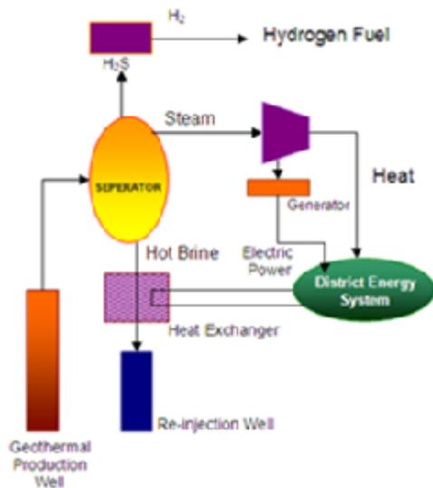
Figure 4. Central geothermal plant layout.
