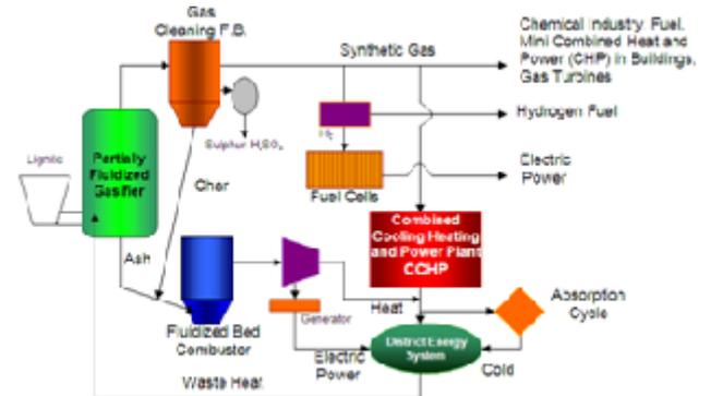
Figure 3. Central plant for clean hybrid lignite utilization system.
