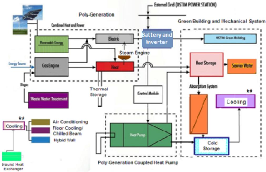
Figure 2. Closed-Loop, High Energy and Exergy Efficiency District Energy Plant
