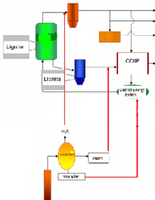
Figure 5. Hybrid clean lignite and geothermal plant coupling for Aydın DE system.
