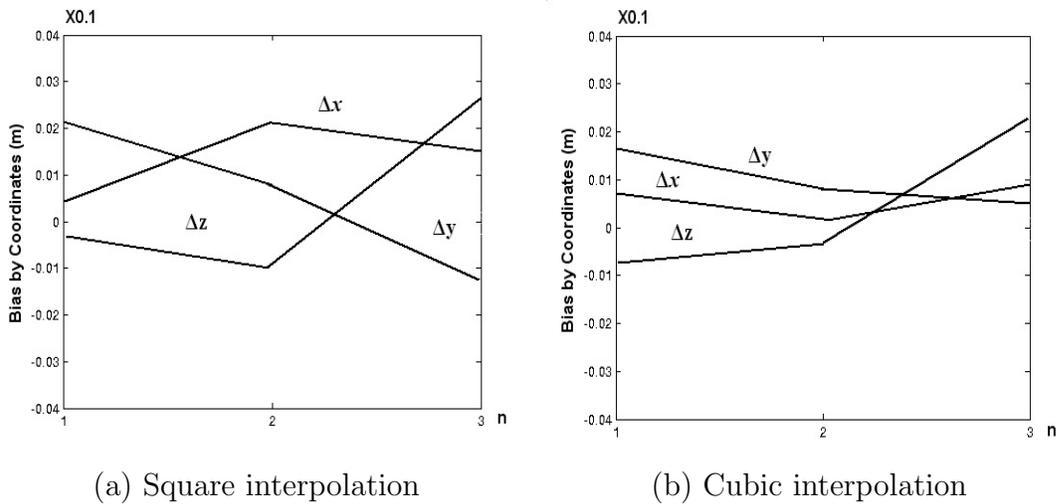
FIGURE 5. The error reduction in measuring of coordinates of a signal source in time domain.
