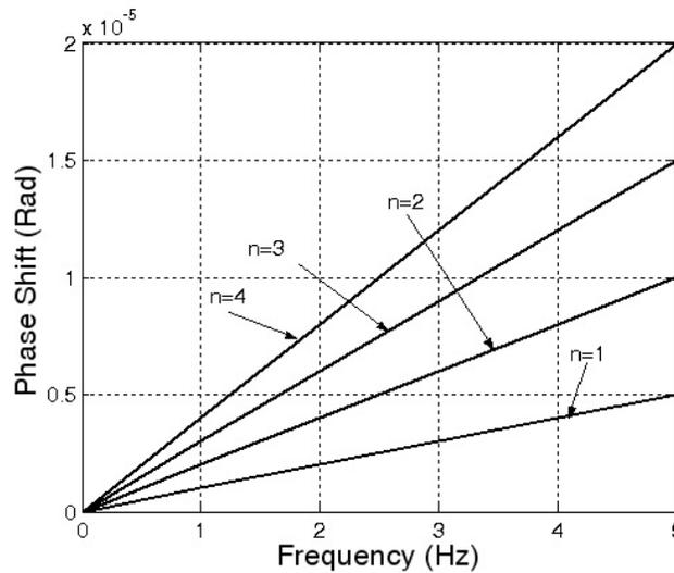
FIGURE 2. The normalized phase shift between adjacent channels for harmonic signal for the range of frequencies from 0 to 5 Hz.
