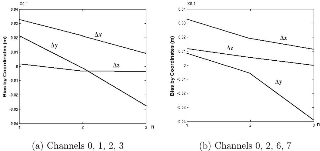
FIGURE 4. The error of coordinates measuring of a signal source for the different sets of the ADC channels.
