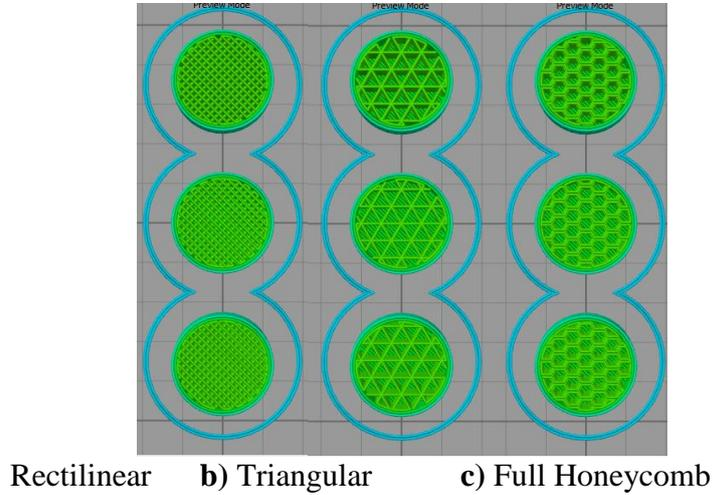
**Figure 2.** Filling structures modeling
