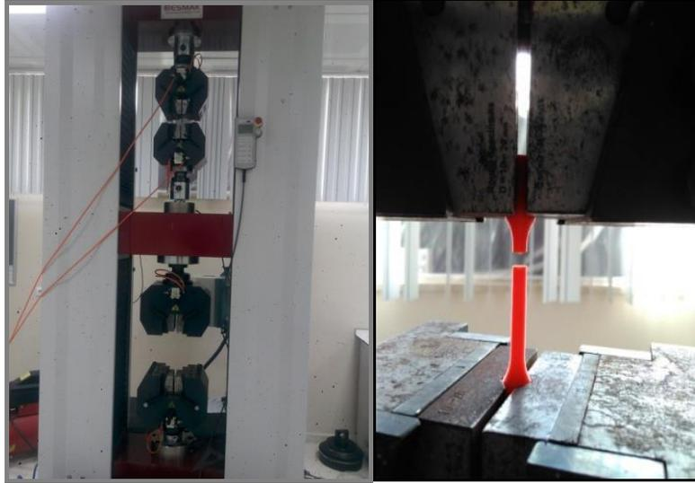
**Figure 5.** Tensile test machine and damaged sample
