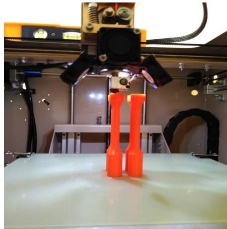
**Figure 4.** Printed standard tensile test samples
