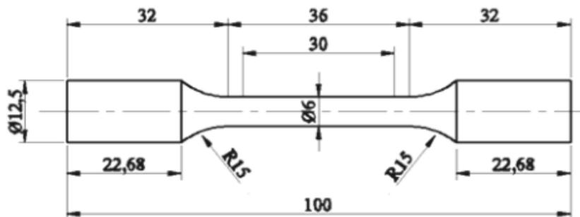
**Figure 3.** Dimensions of standard (TS 138-A) tensile test samples
