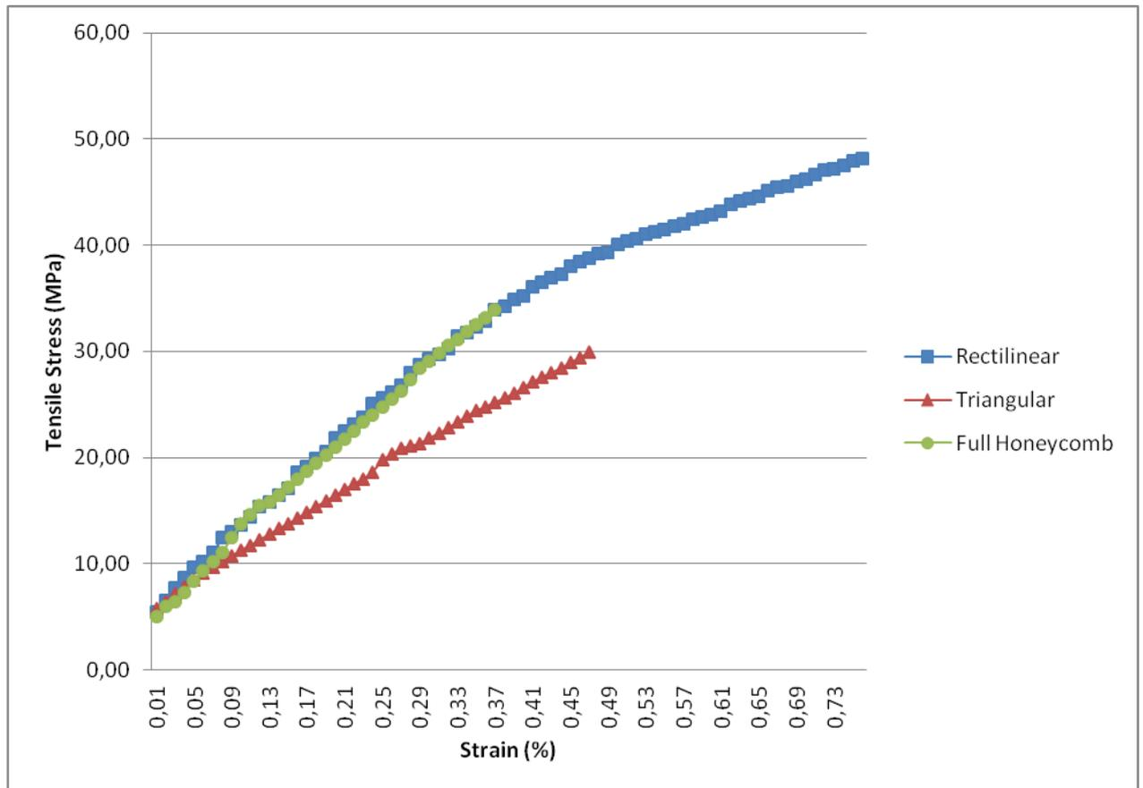
**Figure 6.** Average stress versus strain values for filling structures
