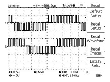
Fig. 9. Line-to-line voltages of VSI
