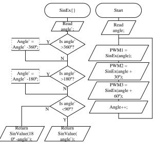
Fig. 4. Algorithm of SPWM signal generation using 3 PWM channels
