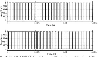
Fig. 7. Modelled SPWM signals for controlling two legs of six-phase VSI
