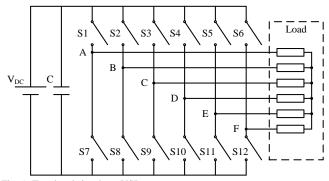
Fig. 1. Two level six-phase VSI
