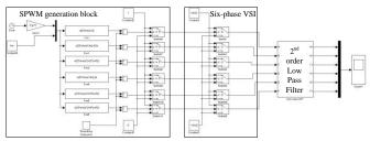
Fig. 5. Matlab Simulink model of idealized six-phase VSI with SPWM control
