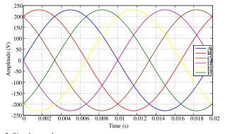
Fig. 3. Six-phase voltage
