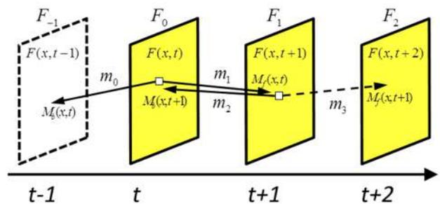
Figure 3. Three frames and one previously estimated motion vector are used to find  $M_f(x, t)$  and  $M_b(x, t + 1)$ .
