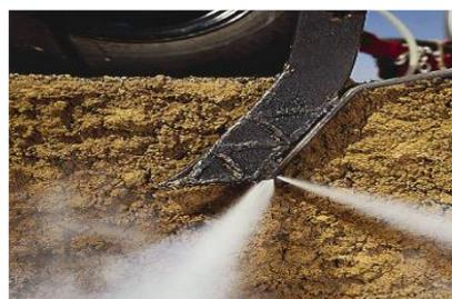
Figure 2. Knife type injection unit
