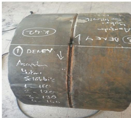
Figure 3. Pipes prepared for welding operation
