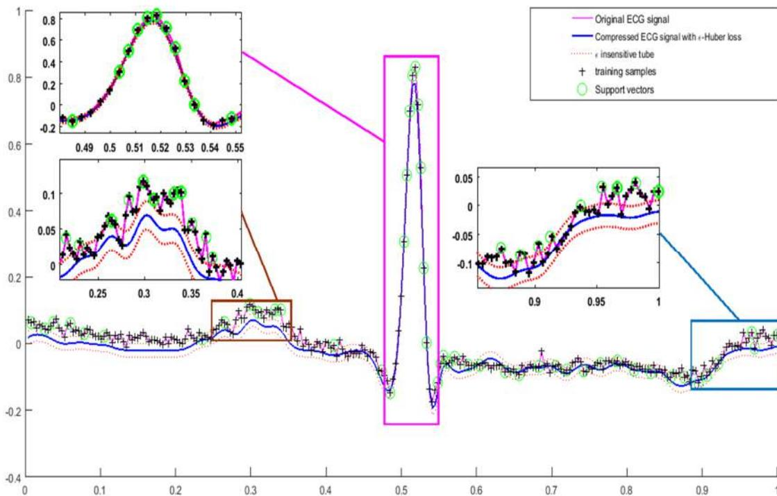
Figure 5. ECG (dark blue) signal compressed by  $\epsilon$ -insensitive Huber loss based SVR. The areas separated by the red dashed line below and above the compressed ECG signal show the  $\epsilon$ -insensitive regions. The '+' signs in the black color represent the training samples, and the '+' signs in the green circles represent the support vectors (the training samples that yield the compressed ECG signal).
