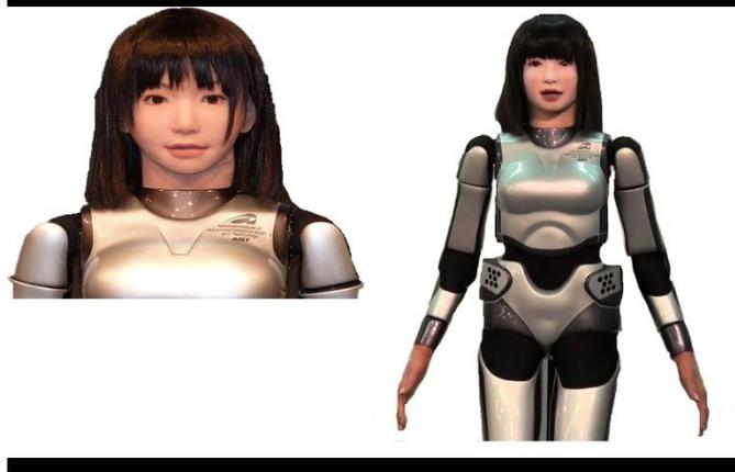
Picture 2 Android Robot HRP-4C
