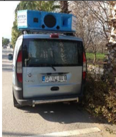
Figure 2. Typical installation of mobile average speed enforcement system (Ilgaz and Saltan, 2017)
