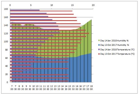
Figure 3. Values of relative humidity (%) and temperature (°C) during two days of experimental testing
