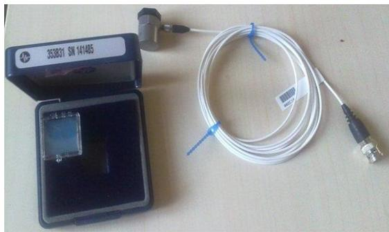
Figure 2. PCB 353B31 vibration sensor
