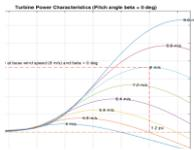
**Figure 3.** Turbine power characteristic for different wind velocity with 8m/s as the base wind speed
