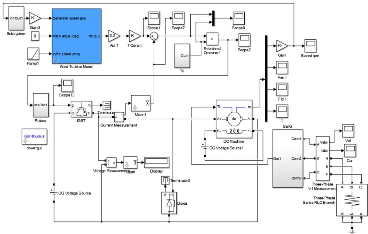
**Figure 2.** Simulink block diagram of wind turbine emulator with SEIG
