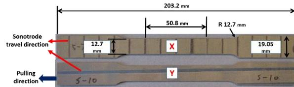
**Figure 3.** Dimensions of the tensile test samples.
