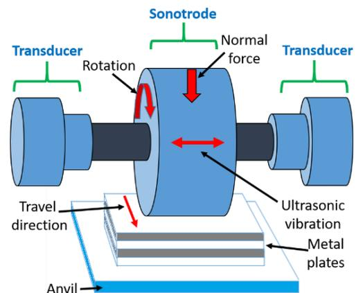
**Figure 1.** Schematic of the ultrasonic consolidation process.
