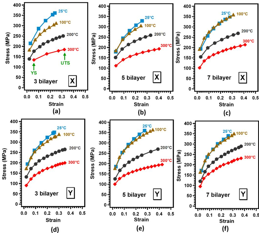
**Figure 5** Stress-strain curves of laminated metal composites obtained from tensile tests; (a to c) X samples, and (d to f) Y samples.
