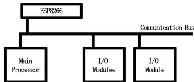
**Figure 3.** How ESP8266 connected to the main processor.
