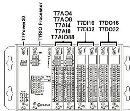
**Figure 1.** T7RIO remote I/O and its modules.
