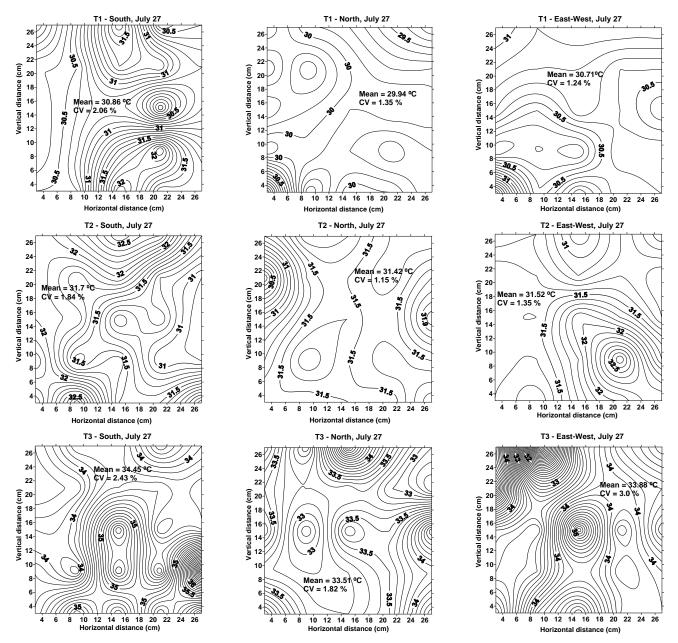
Fig. 1. Kriging curves showing the spatial distribution of canopy temperature (Tc,  $^{\circ}$ C) taken from all cardinal points (North, South and East-West combined) to a 0.3 m x 0.3 m square canopy area by thermal images taken from 1.0-1.5 m distance in all peach irrigated treatments (T1 – T3), the 27<sup>th</sup> of July 2012; note here and in the following graphs that the scales represent the dimensions of the square image
