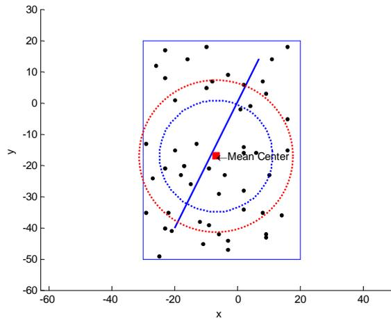
Figure 3. Spatial distribution of geodetic points in simulated earthquake area – meancenter (red square), standard distance (red dashed circle), standard deviational ellipse (blue dashed circle).
