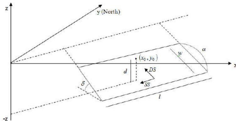
Figure 1. The fault plane geometry.
