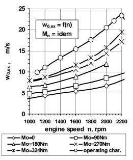
Figure 5. Average velocity  $w_{0,ex}$  of exhaust gas in the converter SZOP 07 – versus engine speed
