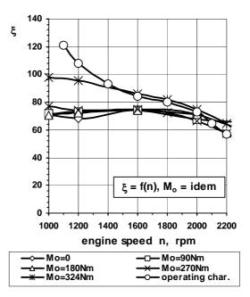
Figure 6. Resistance number  $\xi$  of the catalyst SZOP 07 – versus engine speed
