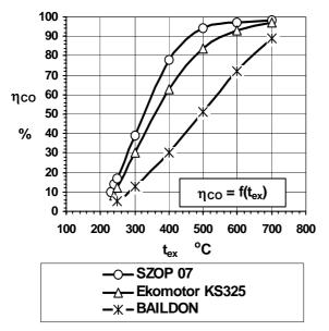
Figure 2. CO conversion efficiency  $\eta_{CO}$  within the oxidation catalytic converters tested – versus exhaust gas temperature  $t_{ex}$
