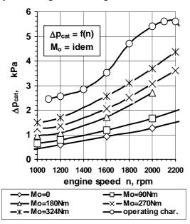
Figure 4. Pressure drop  $\Delta p_{cat}$  within the catalytic converter SZOP 07 – versus engine speed
