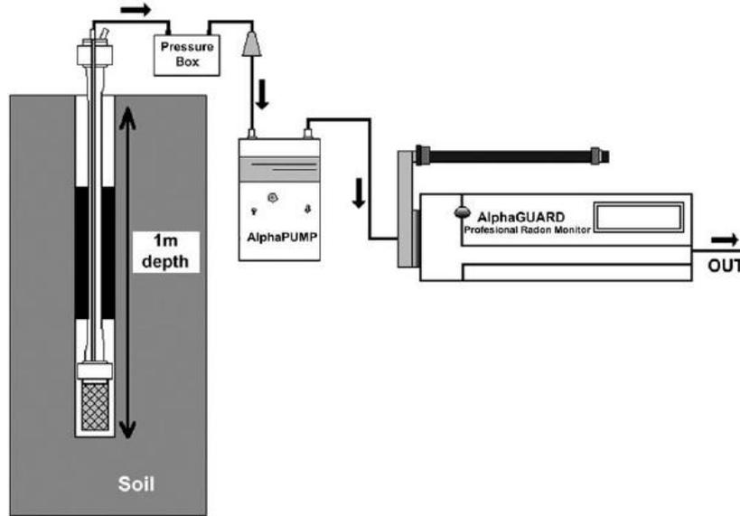
FIG. 2. Schematic view of experimental setup of soil gas radon measurement
