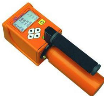
FIG. 1. Portable BGO gamma detector
