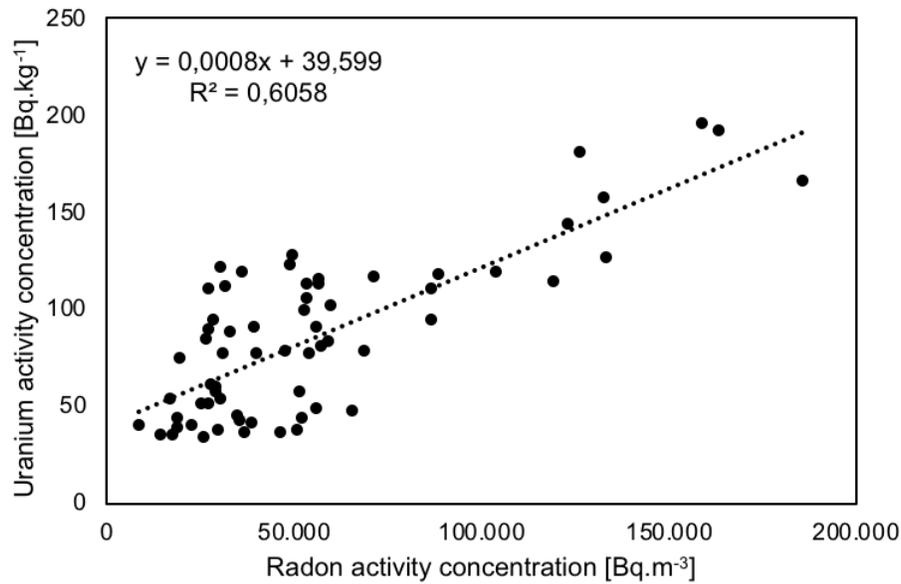
FIG. 3. Correlation of Uranium and radon activity concentrations in soil
