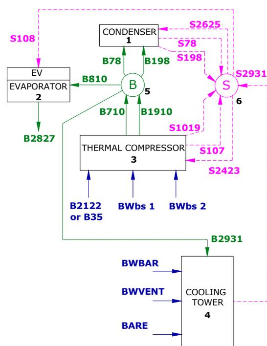
Figure 5. Productive Structure for the Functional Analysis (Double-effect Cycle).
