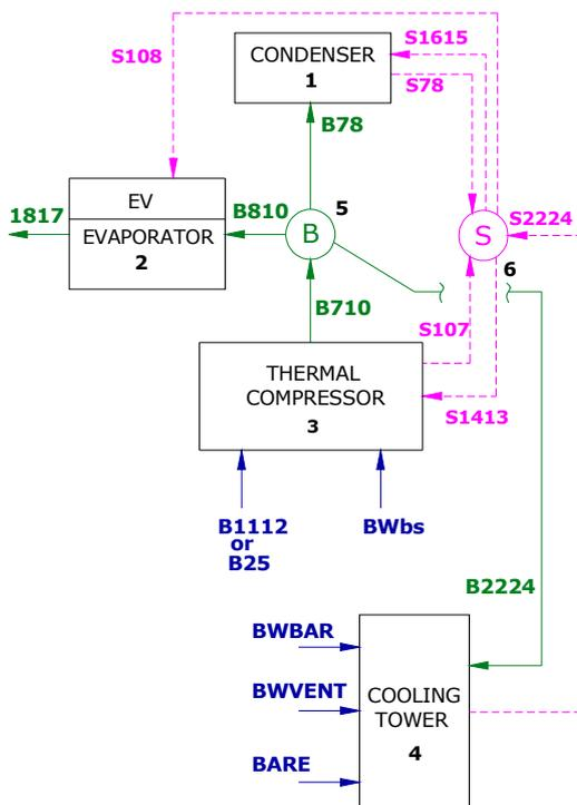
Figure 4. Productive Structure for the Functional Analysis (Single-effect Cycle).
