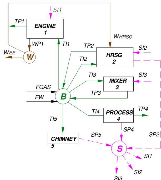
Figure 7. Productive Sstructure for the Functional Analysis of the Cogeneration System.
