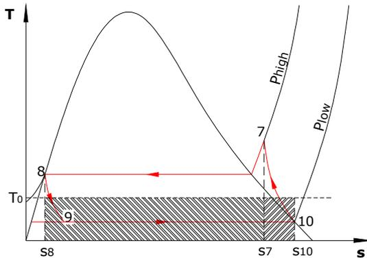
Figure 3. Diagram  $T$ - $s$  for the Water Cycle (Single-Effect Cycle).
