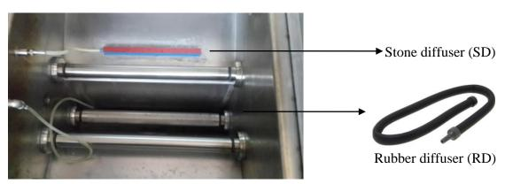
Figure 2. The settlement of the diffusers transferring the ozone gas [20]
