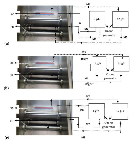
Figure 3. The methods of the ozone feeding to the jigger
