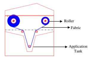
Figure 1. The technical drawing of the jigger machine [20]
