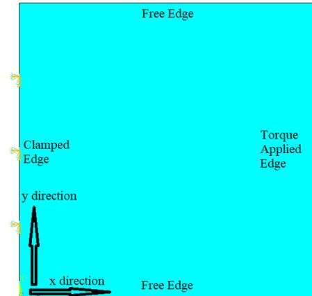
**Figure 3.** Laminated composite plates with C-F-F-F boundary conditions
