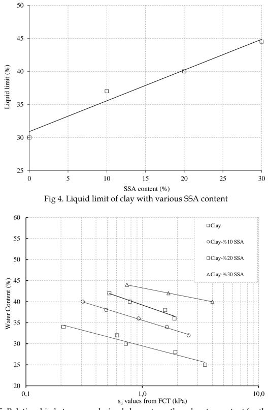
Fig 5. Relationship between undrained shear strength and water content for the clay with various SSA content
