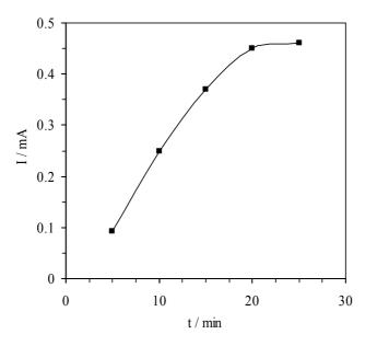
Figure 4. Variation in stripping peak current with time.  $C_{Cu(II)}$ = 0.020 mmol L<sup>-1</sup>, E<sub>d</sub>= -0.70 V
