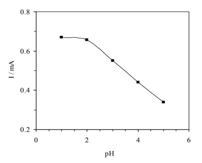
Figure 3. Variation in stripping peak current with pH.  $C_{Cu(II)}$ = 0.20 mmol L<sup>-1</sup>, E<sub>d</sub>= -0.70 V and t<sub>d</sub>= 5 min
