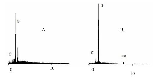
Figure 2. EDX spectrum of a) PAT, b) PAT preconcentrated with copper
