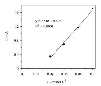
Figure 5. Variation in stripping peak current with Cu(II) concentration at pH=1.0.  $E_d$ = -0.70 V and t<sub>d</sub>= 20 min
