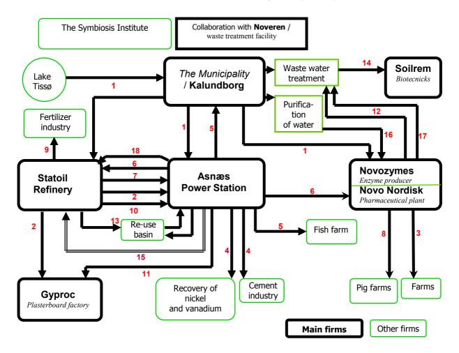
Materials: 1:Surface Water / 2:Gas / 3:Biomass / 4:Fly Ash / 5:Heat / 6:Steam / 7:Cooling Water / 8:Yeast Slurry 9:Sulphure Fertilizer / 10:Tech.Water / 11:Gypsum / 12:Waste Water / 13:Drain Water / 14:Sludge / 15:Deionized Water / 16:Water / 17:Alkoholic Residue / 18: Sea Water
