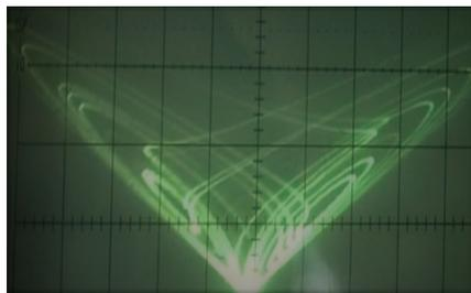
FIGURE 9. y-z phase portrait: CH1(Y) Volts/Div: 0.5V, CH2(Z) Volts/Div: 1V
