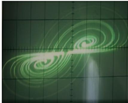
FIGURE 7. x-y phase portrait: CH1(X) Volts/Div: 1V, CH2(Y) Volts/Div: 2V
