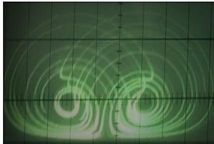
FIGURE 8. x-z phase portrait: CH1(X) Volts/Div: 1V, CH2(Z) Volts/Div: 2V
