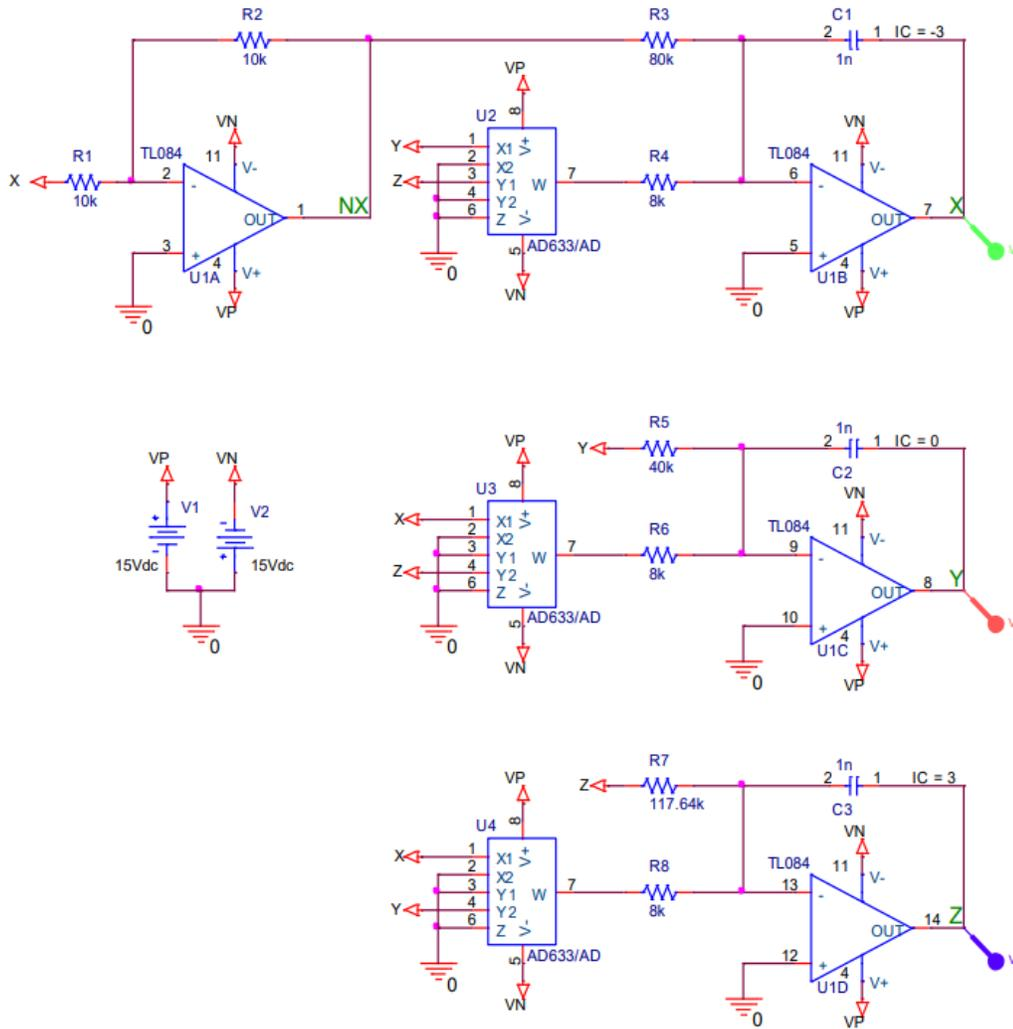
FIGURE 5. Schematic of the designed electronic oscillator of the Lu - Chen system
