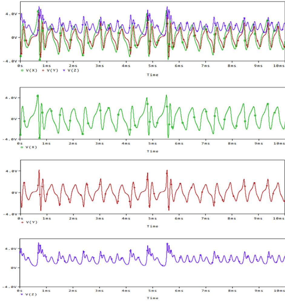
FIGURE 6. x-y-z signals from the PSpice simulation of the Lu-Chen oscillator
