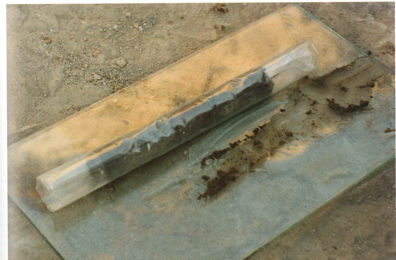
Figure 2: Pollen core sample consolidated by wrapping with plastic
