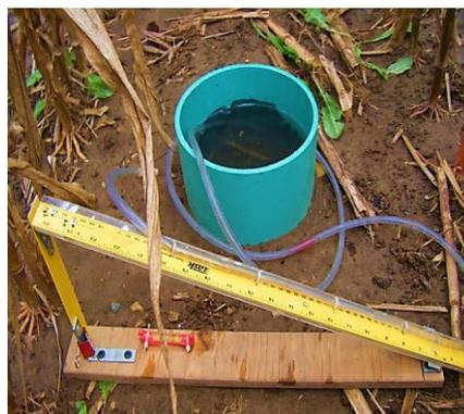
Plate 1. Set up of infiltration apparatus
