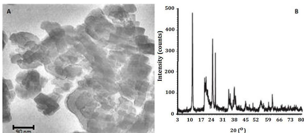
Figure 1. (A) TEM image and (B) XRD pattern of applied nanozeolite
